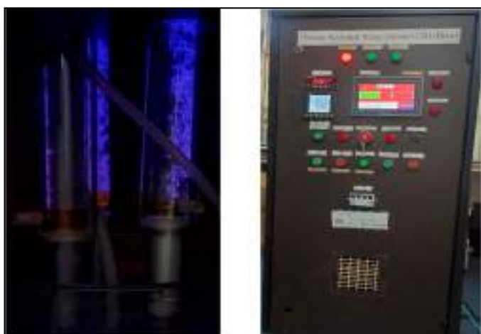
Figure 3: PAW generation system and its control unit
