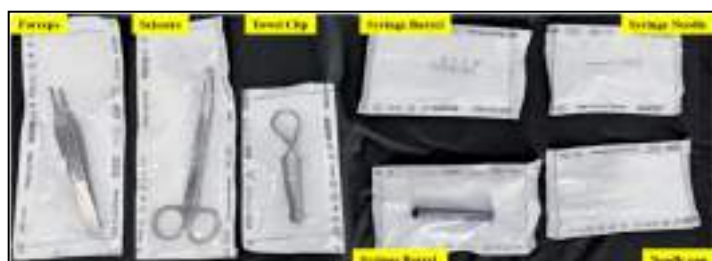
Figure 4: Tyvek sealed surgical equipment loaded with Staphylococcus aureus (SA) bacteria
