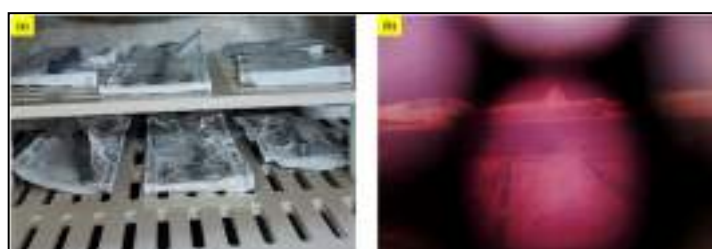
Figure 5: (a) Tyvek sealed surgical equipment inside sterilization chamber (b) equipment getting exposed to plasma
