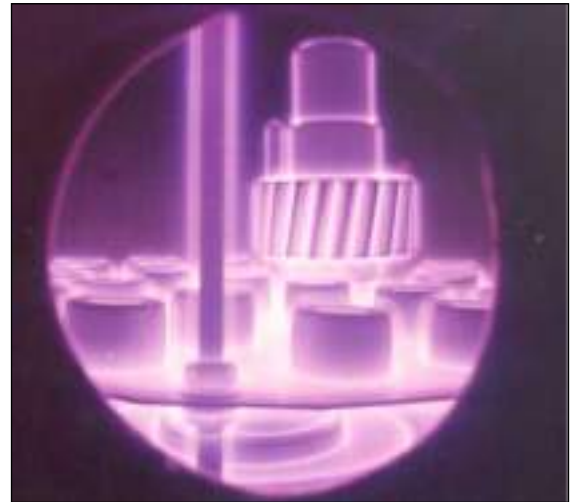
Figure 1: Plasma glow around gears and other components during plasma nitriding
